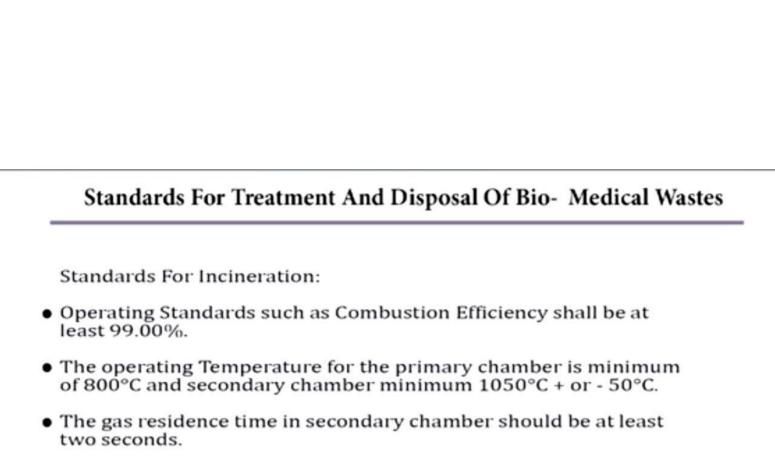
Emission Standards: For Particulate matter, Nitrogen Oxides (NO) and hcl, Dioxins and Furans and Mercury (Hg) and its compounds.
